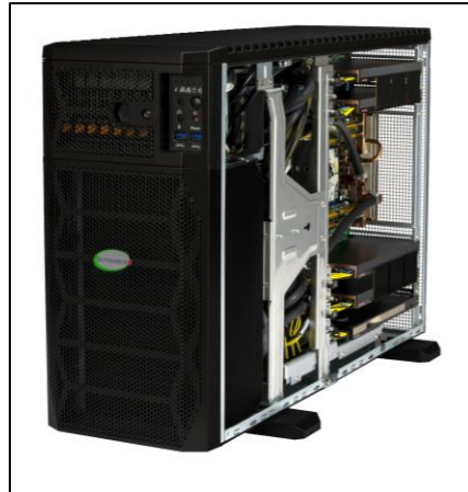
Figure 7 - Open Side View of Liquid Cooled System
